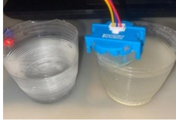
Gambar 11 Implementasi sensor Turbidity
