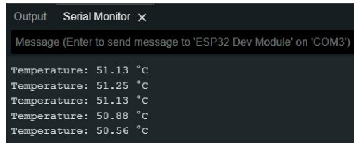
Gambar 8 Serial monitor Sensor ds18b20
