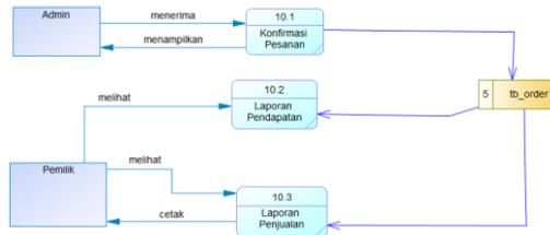
**Gambar 6. DFD Level 1 Proses Laporan**
